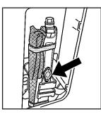
Install the jack in the driver's side panel of the rear cargo area and secure with the wing bolt.
